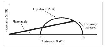
**Figure 1.** Geometric mapping projection of the dependency between phase angle ( $\varphi$ ) and resistance (R), reactance (Xc), impedance (Z), and the frequency of the current.
